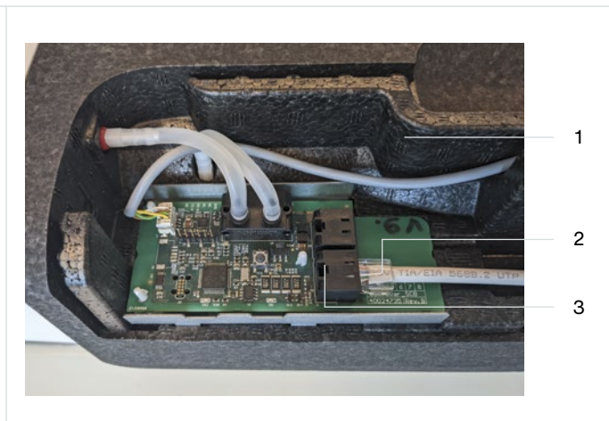
Fig. 5.10 – RJ45 sockets VM-PCB
