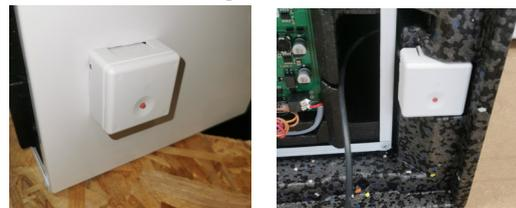
5. Insert the plug of the connection cable into the socket of the control board (see electrical connection) and place the cable in the cable guide provided. The remaining cable is kept in the space between the EPP housing and the metal housing.
