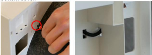
3. Press the connection cable into the cable recess of the EPP housing and close it again with the adhesive tape. Using a suitable pair of flat-nose pliers, separate the cut-out for inserting the connection cable into the housing of the radio module.
