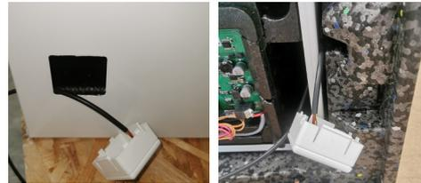
4. For wall or ceiling installation, clip the radio module into the break-through opening of the metal housing while pressing the locking connections together lightly. For mounting in a flush-mounting box, place the radio module in the cut-out in the flush-mounting box.
