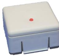
If the LED lights up **green**, the ventilation unit is still in another network or is networked with another unit. This networking must be cancelled before you can add the unit to a network in the app. To cancel the network, press and hold the red button while the green LED is lit until the LED lights up **white** (approx. 10 seconds). Now you can continue registering the ventilation unit in the app.
