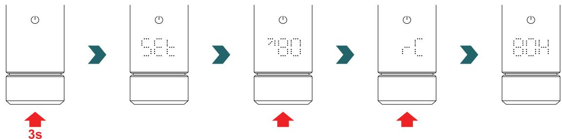
While “BOX” is displayed turn the rotary knob to initiate the pairing process.
