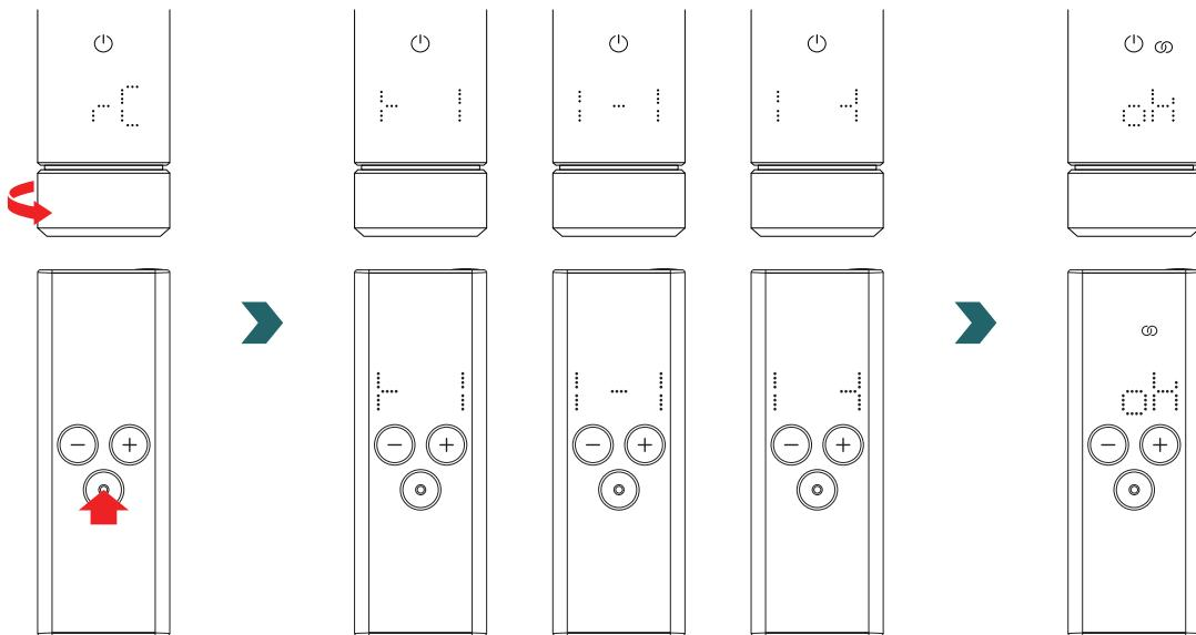
While “rC” is displayed turn the rotary knob. The pairing process starts for 60s, during this time press any button on the RCE.
